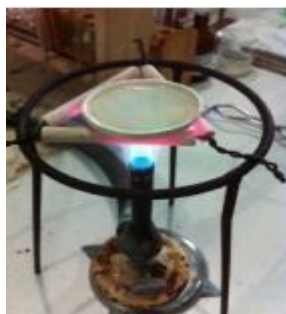
Figure 3. SnO 2 F deposition tool set using the burner Bunsen
