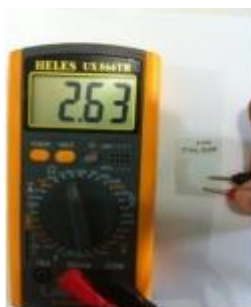
Figure 4. Measurement of the resistance of the resulting FTO glass sheet by using the AVO meter
