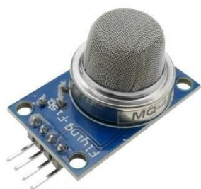
Gambar 3. Sensor Gas MQ-02 (Sumber : www.arduino.cc )
