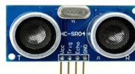
Gambar 2. Sensor Ultrasonic HC-SR04 (Sumber : www.arduino.cc )
