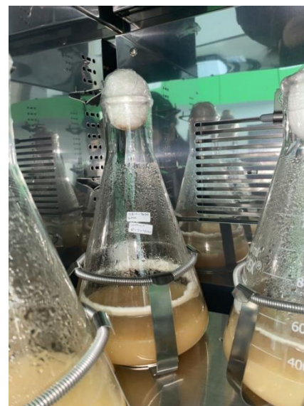
Figure 2. Rhizosphere isolates of Fusarium sp. LBSU fermented in a shaker incubator for 21 days at 30°C
