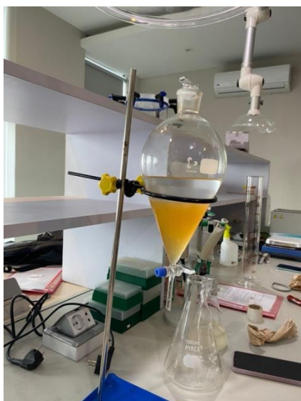
Figure 3. The extraction process of secondary metabolites from liquid fermentation media of rhizosphere isolates of Fusarium sp. LBSU
