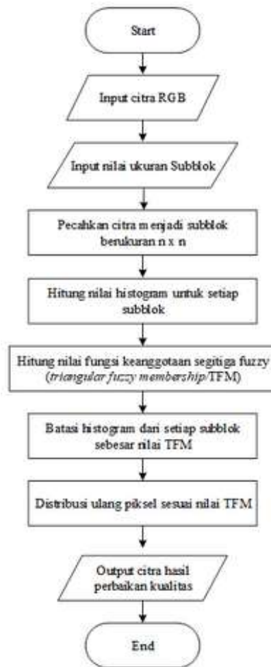
Gambar 3. Flowchart Triangular Fuzzy Membership-Contrast Limited Adaptive Histogram Equalization (TFM-CLAHE)
