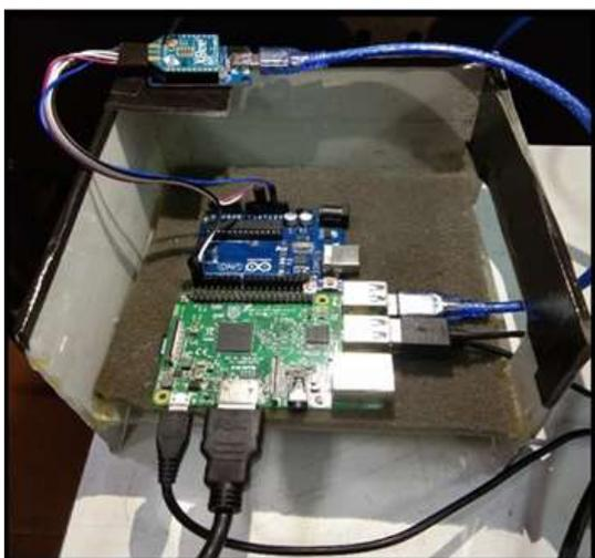
Figure 16 Xbee receiver
